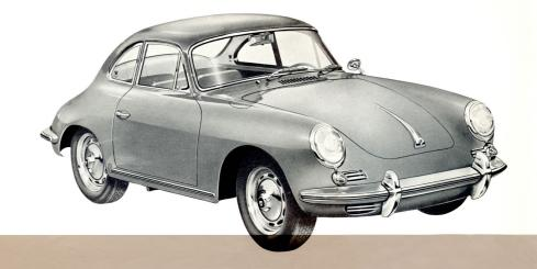
The fresh-air vent below the panoramic windshield furnishes fully controlled ventilation to the passenger compartment.
