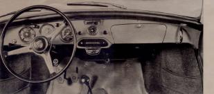
All models for 1962 have a new redesigned instrument panel with improved instrument positions.
